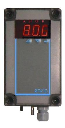
The DP-101SPD is a surface mounting meter with a 4 digit numerical display intended for the measurement of pressure differences. The measurement unit also has a square root function which allows the display and the output to be scaled in pitot tube measurements to give the flow volume. It is delivered with a built-in sensor and is pre-programmed ready for use.
