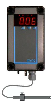
The DP-101S-AF is a surface mounting meter with a 4 digit numerical display intended for the measurement of air-velocity in air-conditioning, clean room, fume hood etc. applications. The measurement unit also has an area x air-velocity calculation function which allows the display and the output to be scaled in air-velocity measurements to give the flow volume. It is delivered with a built-in sensor and is pre-programmed ready for use.
